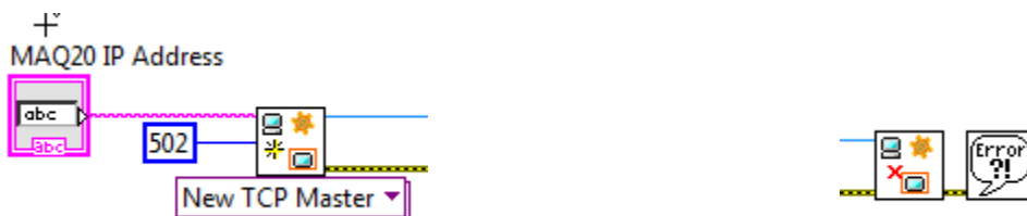
Figure 1: Modbus TCP VIs
